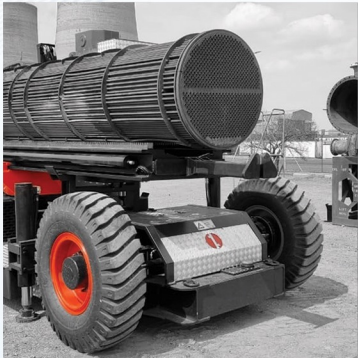
HEAT EXCHANGER/BUNDLE HANDLING
