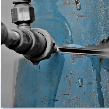
ABRASIVE COLD CUTTING
